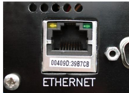
RJ45 Ethernet connector 8P8C (B) at valve controller
